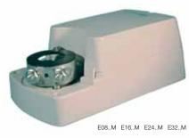
Motor stops automatically when in the end position. Up to 5 motors can be wired in parallel. Max. ambient -20/+50°C Adjustable angle of rotation limiter 0-90° Reversible position indication 0-10, 10-0 Noise level 45dB Latchable Manual Override Supply : 24VAC ±20% 24VDC ±10% 230VAC ±10% 24V=7.5VA 230V=6VA Enclosure Flammability = UL94-V0
