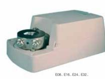
Up to 10 motors can be wired in parallel. Max. ambient -20/+50°C The motor stops automatically when the end positions are reached. Angle of rotation 0-90° adjustable Reversible position indication 0-10, 10-0 Noise level 45dB Manual Override Supply : 24VAC ±20% 24VDC ±10% 230VAC ±10% 24V=6.5VA 230V=6VA Enclosure Flammability = UL94-V0
