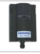
Do not expose to extreme ambient or oily/dirty conditions. 24VAC supply, green power led. Red led and sounder alarm. Volt free alarm relay rating 1A-Factory set threshold. Analogue output 0 to 10VDC or 4-20mA Dimensions 86x120x53 180gm Standard housing IP41
